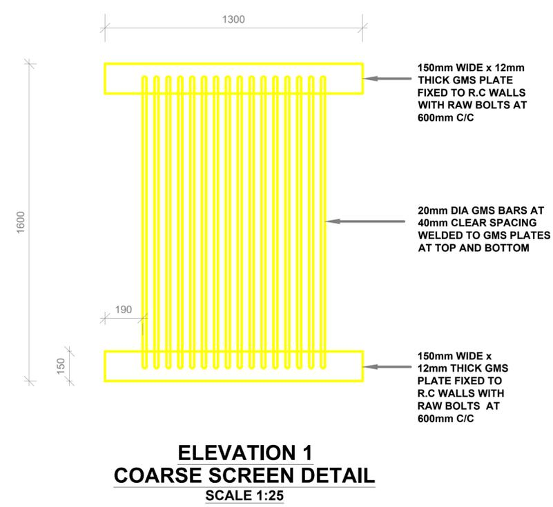
**ELEVATION 1 COARSE SCREEN DETAIL**
